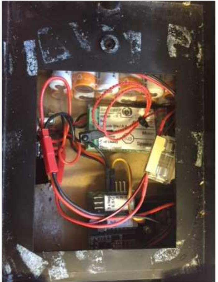
This is the view of the card to which all the components are fixed (the coal load has been removed). The tender body has to be removed to install the components. If you look closely in the centre the 'magic eye' can be seen (black item on end of red cable).
